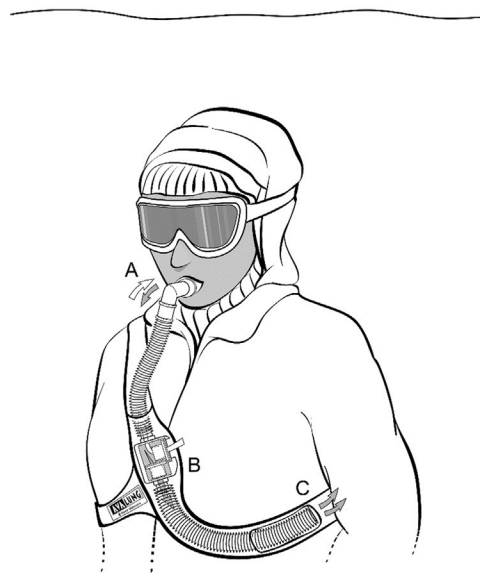
Figure 3. The artificial air pocket device that diverts expired air away from inspired air during avalanche burial is intended to prolong survival of fully buried avalanche victims. The white arrows show the flow of inspired air, and the gray arrows show the flow of expired air.
